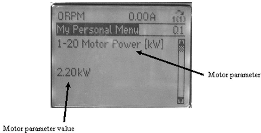
**My personal menu** These are the user modifiable parameters that are used when setting up the Milkflow controller such things as motor power, automatic motor adaptation, motor ramp times, low and high speed limits etc...
